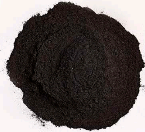
Graphite powder recovered from industrial production of electrodes
